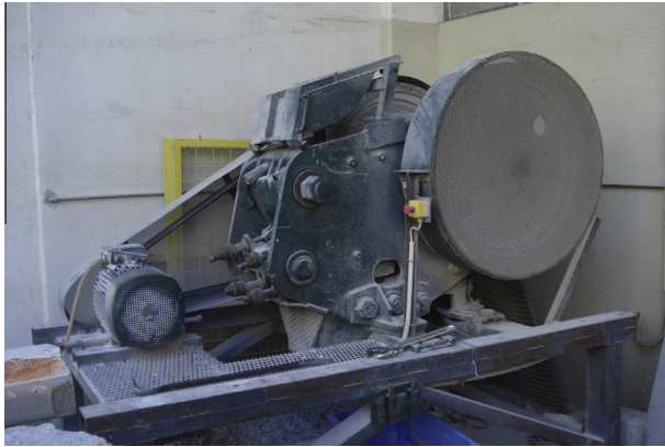
Fig. 1. Primary crushing equipment: impact crusher.
