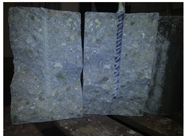
Fig. 5. Vertical cracking plan of the specimen.
