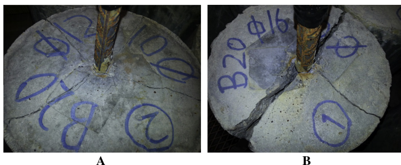
Fig. 12. Failure modes vs. steel rebar diameter.
