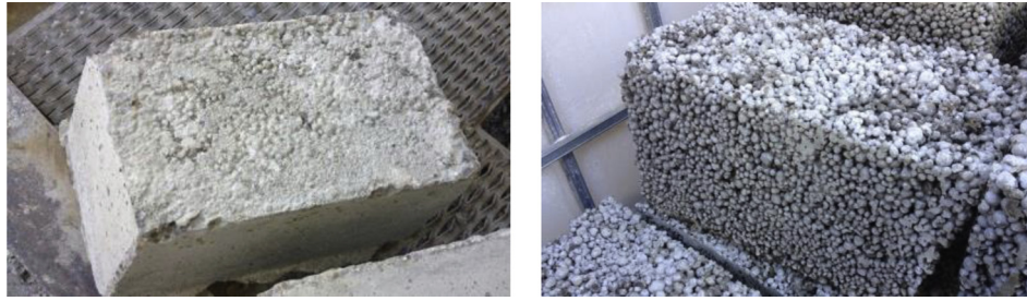
Fig. 1. Original structural LWCHD (left) and no-fines non-structural LWCM (right).
