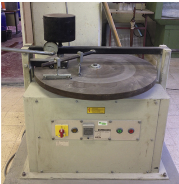
Fig. 3. Abrasion test according to DIN 52108 (2002).
